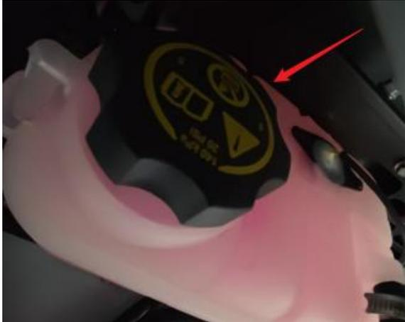
A close-up photograph of the black plastic cap of the coolant reservoir. The cap has a yellow warning symbol and text. A red arrow points to the cap, indicating it should be unscrewed.                                                                                        |
