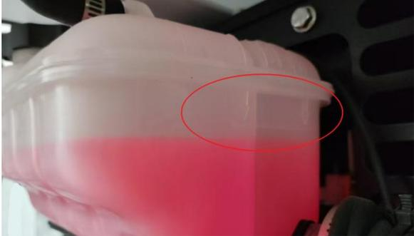
A photograph of a white plastic coolant reservoir. The reservoir is partially filled with pink coolant. On the right side of the reservoir, there is a vertical scale with a minimum level mark. A red oval highlights this mark and the coolant level, which is below the mark. |
